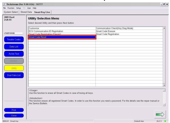
6. Make sure driver door is open. Other doors must be closed. Don't touch steering wheel and pedal.
