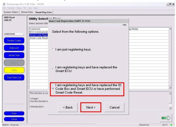
3. Program keys. To register key touch the Power/Engine Switch with the key – you will hear a signal, and then move the key to the center of car cabin – you will hear a signal once again. To register second, third key, etc. – just repeat "touch and move" operations. You have 30 seconds to do this.
