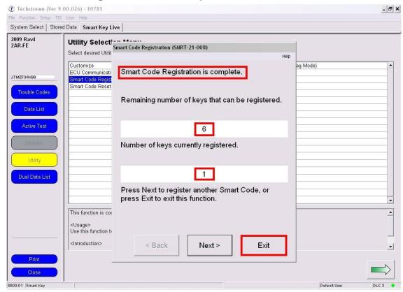
IMPORTANT! You can use this **Smart Code Registration** procedure even **ID Code Box** and **Smart ECU** had **not** been replaced. Both for new and used smart-keys.
