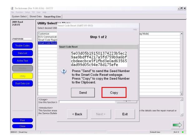
8. Open PASS-CODE Calculator. Paste VIN vehicle, Seed Number and press Calculate. You will get Pass-Code Number. Paste Pass-Code, click "Next" and confirm:
