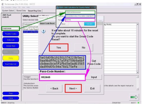
9. **Smart Code Reset** will start. Wait for **16 Minutes** for Smart Resetting. Then use one of the Toyota factory procedure for programming keys.
