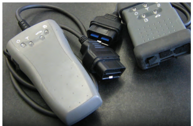
The C-III plus Vehicle Interface (VI) (right) works only with the new software, and is not interchangeable with the basic CONSULT-III VI (left).
